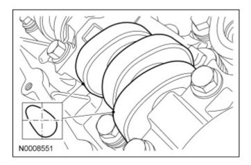
5. NOTICE: If the components are to be reinstalled, they must be installed in their original positions. Mark the components for installation into their original locations. Failure to follow these instructions may result in engine damage.
